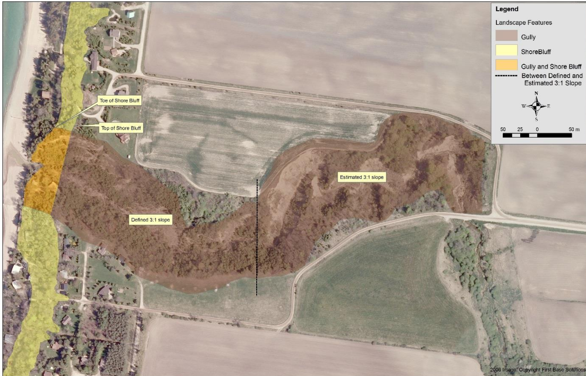
Figure 2.10. Example of shore bluff and gully landforms
