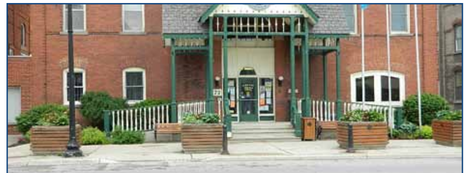
Planters are placed on the landscape strip between the sidewalk and road. Note also the accessibility ramps that are integrated into the front of the municipal offices in Seaforth, but do not obstruct the sidewalk.
